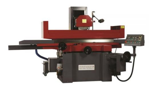
The Brenner RAD Rapid Feed Surface Grinding Machines are produced with highly rigid cast iron body ensuring maximum rigidity. Both the longitudinal and cross feeds are automatic while the vertical feed is manual with a rapid feed function. They are designed to operate with low vibration, high accuracy and low maintenance requirements and include centralised one-shot lubrication. A permanent magnetic chuck, coolant system and a halogen working light are all standard equipment.
