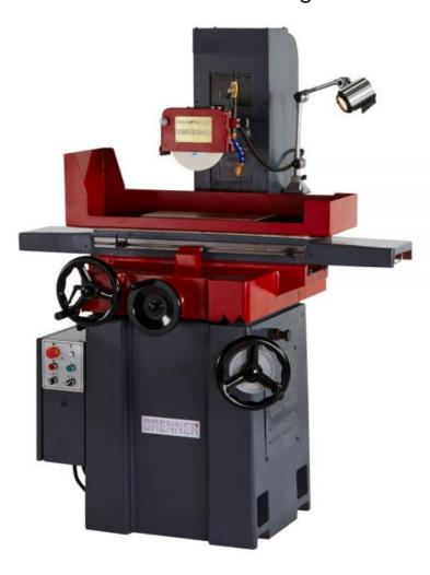
The Brenner 618M Manual Surface Grinding Machine is produced with highly rigid cast iron body ensuring maximum rigidity. It is designed to operate with low vibration, high accuracy and low maintenance requirements and includes centralised one-shot lubrication. A permanent magnetic chuck, coolant system and a halogen working light are all standard equipment.
