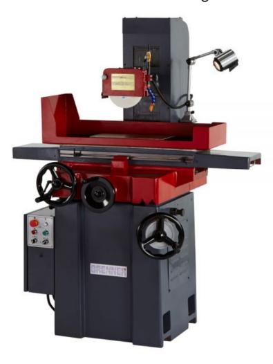
The Brenner 618MB Manual Surface Grinding Machine is produced with highly rigid cast iron body ensuring maximum rigidity. It is designed to operate with low vibration, high accuracy and low maintenance requirements and includes centralised one-shot lubrication. A permanent magnetic chuck, coolant system and a halogen working light are all standard equipment.
