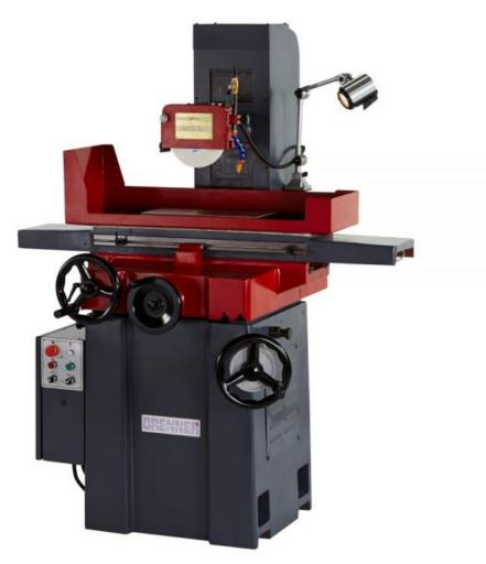
The Brenner 820 M Manual Surface Grinding Machine is produced with highly rigid cast iron body ensuring maximum rigidity. It is designed to operate with low vibration, high accuracy and low maintenance requirements and includes centralised one-shot lubrication. A permanent magnetic chuck, coolant system and a halogen working light are all standard equipment.
