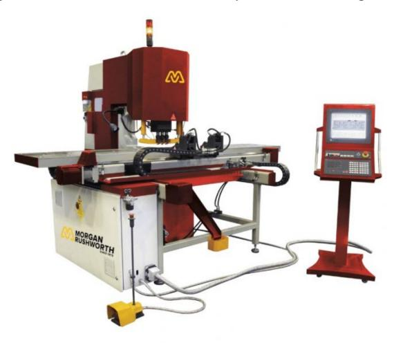
The Morgan Rushworth HSP CNC Punch Range is a high production solution for batch run manufacturing. This 2-axis linear rail and positioning system enables the operator to perform punching operations with no marking or measuring. Once the CNC control has been programmed, the positioning system moves to punch positions with speed and accuracy while multiplying the productivity of the operator. Available on the HSP 95, 125 and 175 punches, this solution will increase production and lower costs
