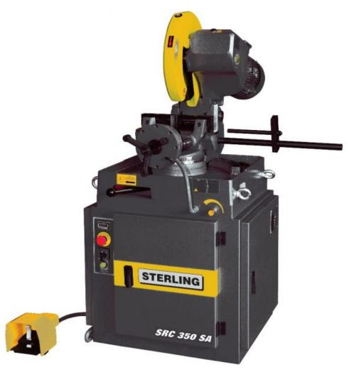
The heavy construction and quality finish of the Sterling SRC range of circular sawing machines is outstanding. Models with 275, 315 and 350mm diameter blades are offered as not only the standard pull down version – with or without a pneumatic vice system – but also in a fast cutting semi-automatic design for production cutting. Double clamping and self-centring vices ensure material is always securely clamped in the optimum cutting position.
