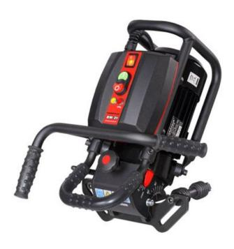
The BM-21 is a bevelling machine designed to bevel materials made of carbon steel. The machine can bevel plates, as well as pipes with outer diameters of 150–300 mm, at an angle of 0–60° and with the bevel width of up to 21 mm. Additionally, the machine contains dampers to reduce vibrations. When equipped with an optional guide, the machine can bevel pipes with outer diameters of 300–600 mm.
