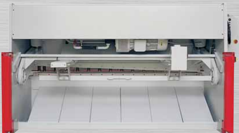
BHGS REAR VIEW INDICATING POWER BACK GAUGE WITH SWING AWAY FEATURE
