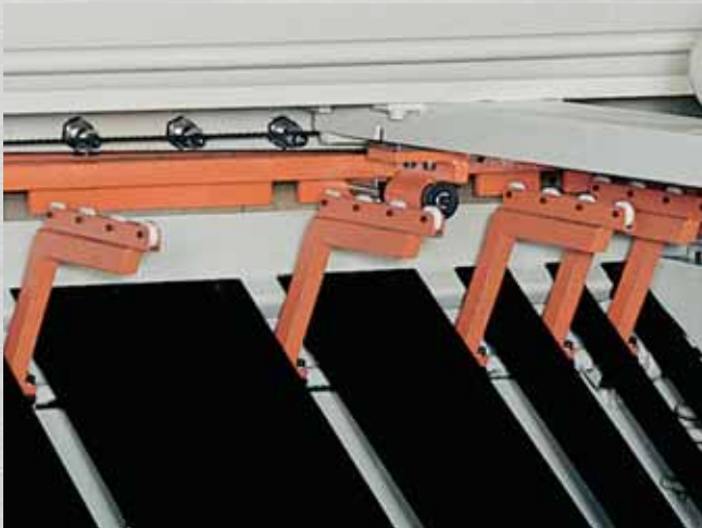
REAR VIEW WITH MOTORISED BACKGAUGE AND OPTIONAL PNEUMATIC SHEET SUPPORT SYSTEM
