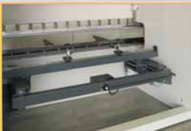
STANDARD REAR CNC REAR BACK GAUGE WITH FINGER DETAIL
