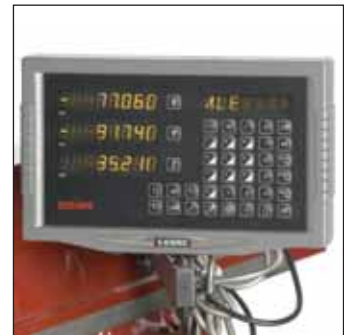
DRO CONTROL PANEL
