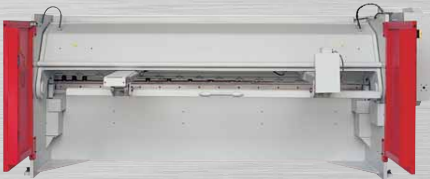
HSGS REAR VIEW WITH POWER BACK GAUGE WITH SWING AWAY FEATURE
